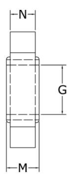
$\begin{aligned} G &= 30 \\ M &= 20 \\ N &= 15 \\ Nom. torque NM (Tkn) = 95 \end{aligned}$
